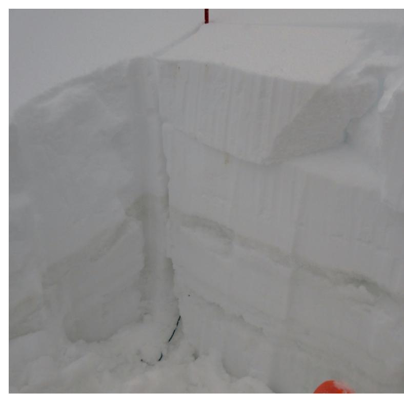
Avalanches were failing within the new snow and this pit had unstable test reuslts (ECTP4) at the same depth. There was a 3" thick supportable crust below the new snow. However, weak, wet snow produced unstable test scores with an ECTP22 on weak, wet depth hoar near the ground. Photo: GNFAC
