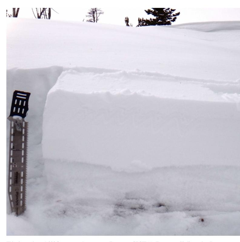
This pit was dug at 9,200 feet on a northeast aspect. Test score of ECTP11. Facets are still alive and well on higher elevation, more east to northersly slopes. Snowpit profile is here:http://www.mtavalanche.com/images/13/snowpit-beehive-basin?size=\_original
