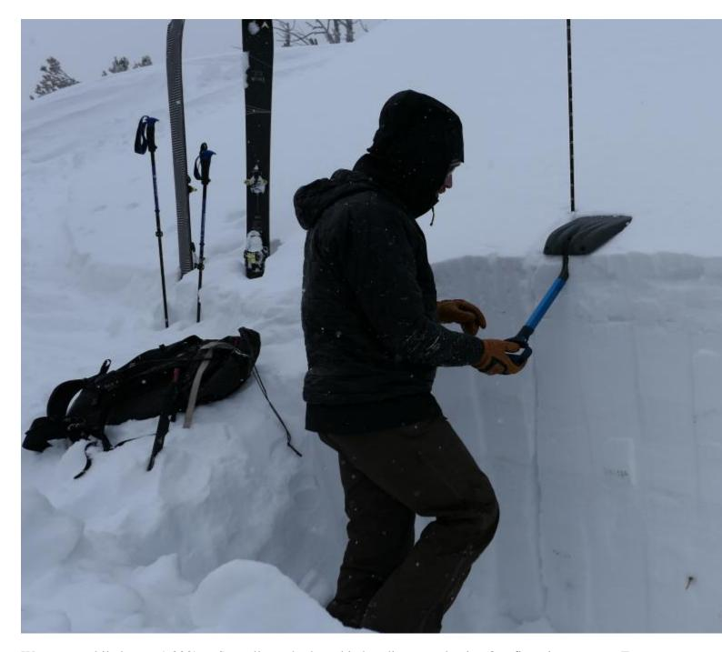
We snowmobiled up to 9,000' on Sawtelle peak, then skied to dig a couple pits. Our first pit was on an East aspect on a heavily wind loaded slope. The HS was 130cm (or 4.2 feet). There was 8" of new snow equal to 0.85" SWE, sitting over old consolidated snow that made up a slab over soft, weak facets about 50cm off the ground. We had ECTP24 x2 break on the old weak snow.... Photo: GNFAC
