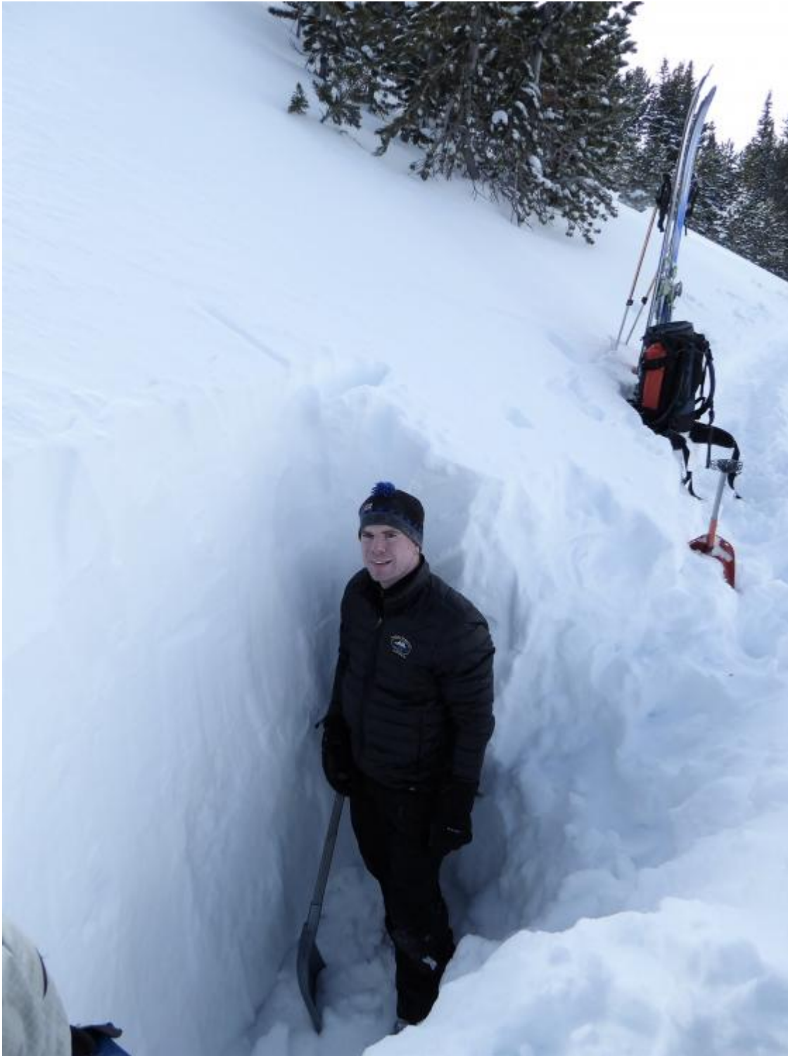
Mike Thom, Gardiner District Ranger, stands in a 7-foot deep snowpit at 9900' on Woody Ridge to the south of Cooke City. We found wind-loading to be our primary concern. Facets were still present at the base of the snowpack, but they are stable for now. Photo: GNFAC
