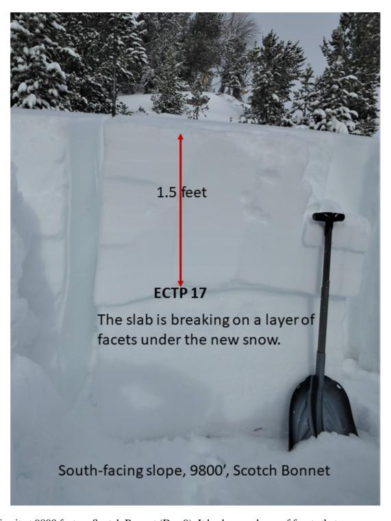
Outside Cooke City we dug this pit at 9800 feet on Scotch Bonnet (Dec 9). It broke on a layer of facets that formed a few days before Thanksgiving and is now buried under 1.5' of snow. The recent storm made this layer reactive. Photo: GNFAC
